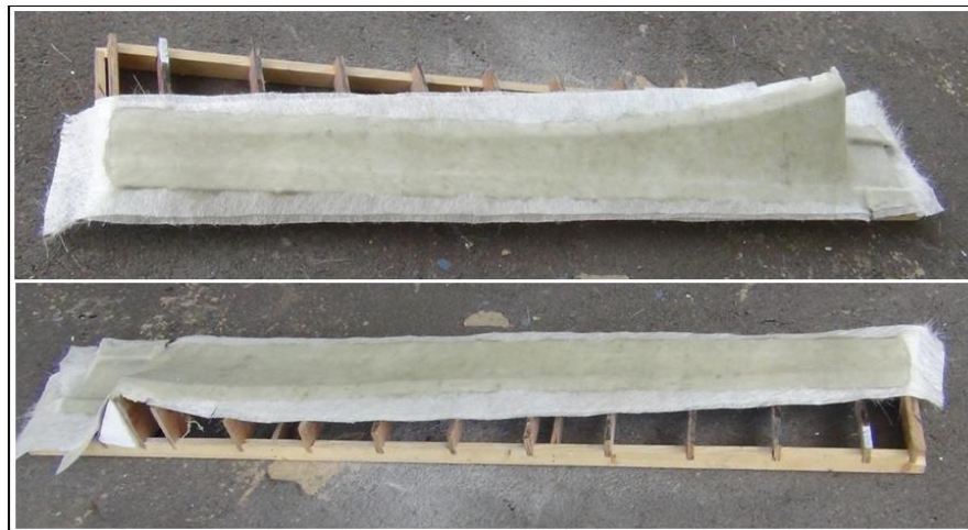
Figure 14. Layers of fiberglass and resin placed to make the two shells of blade.
