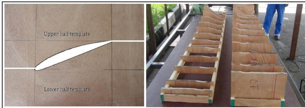
Figure 12. Upper and lower halves of the mold.
