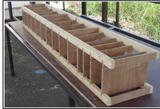
Figure 11. Wind turbine blade mold (templates fixed in their respective position).
