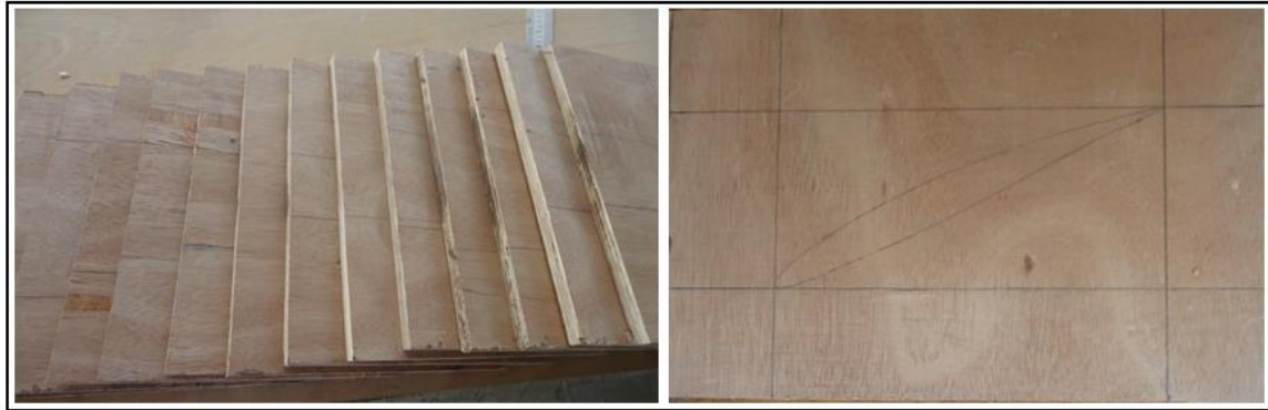
Figure 9. Twelve wooden templates made of plywood of 9 mm thickness.
