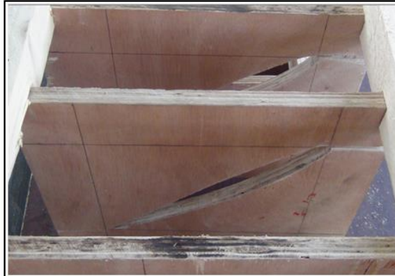
Figure 10. The two elements of the mold (upper and lower halves of the mold).
