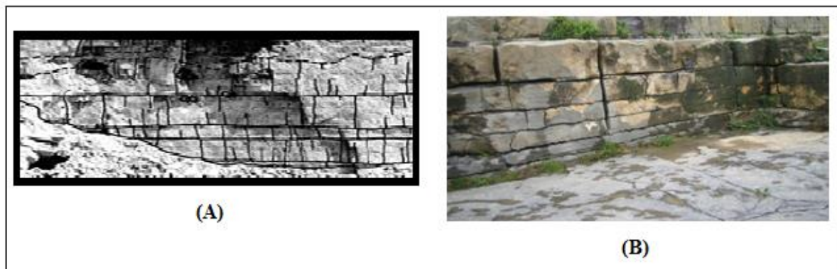
Figure 2. A) Thinly bedded and intensive laterally as well as vertical jointed limestone; B) scarcely vertical and lateral jointed and fractured limestone.
