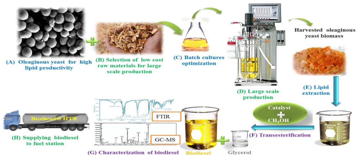
Fig 2. Schematic diagram of biodiesel production from the oleaginous yeast (Patel et al. 2016).
