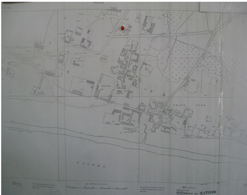
Figure 2: 20th century map of the Ada Foah coastline. Note the red pointer which marks the fort's previous location. The remaining area leading from the south to that marker has been eroded by the ocean (source: Dredging, Environmental and Marine Engineering)
