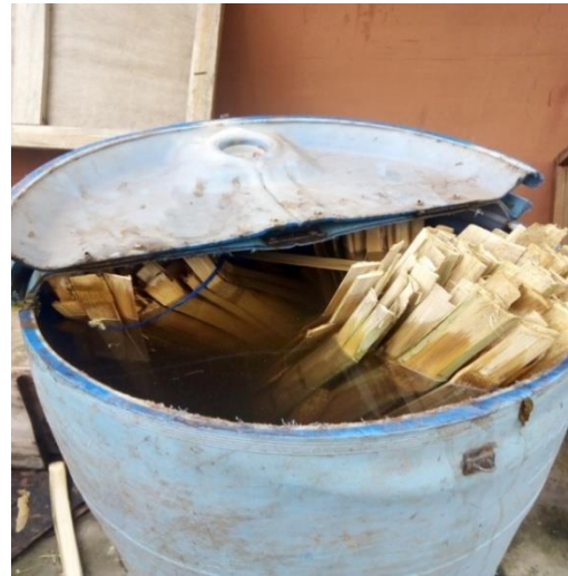
Figure 5: Treatment in Boric Acid solution
