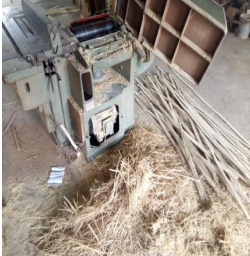
Figure 4: Knot removal and planning
