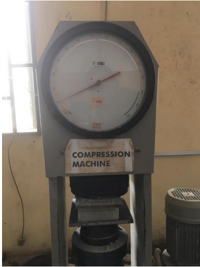
Plate 1: The Compression Testing Machine
