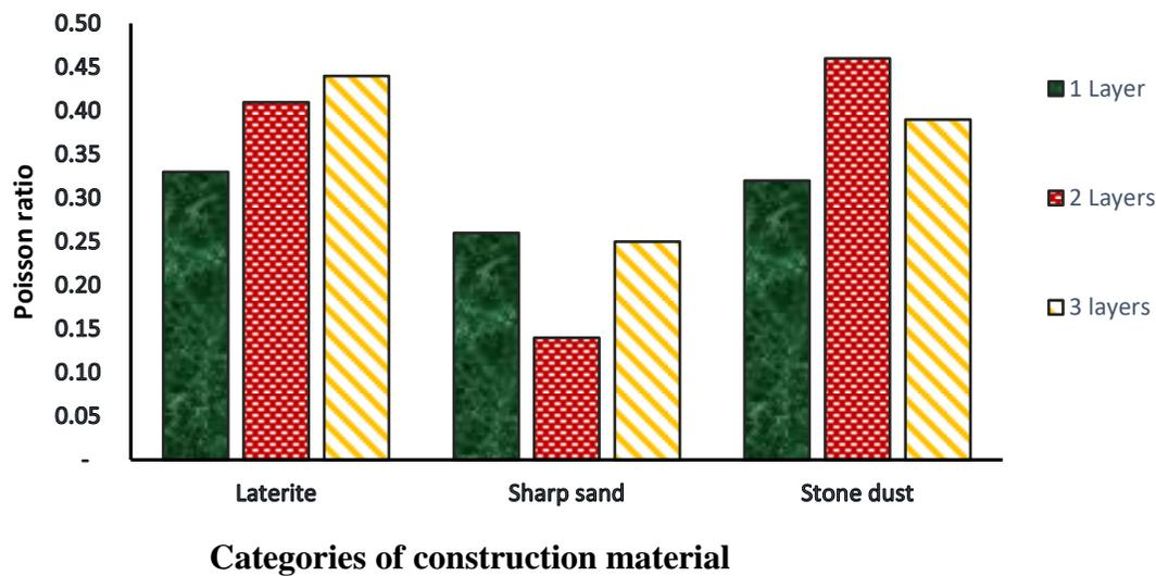
**Figure 5:** Poisson's Ratio of Bottle Bricks
