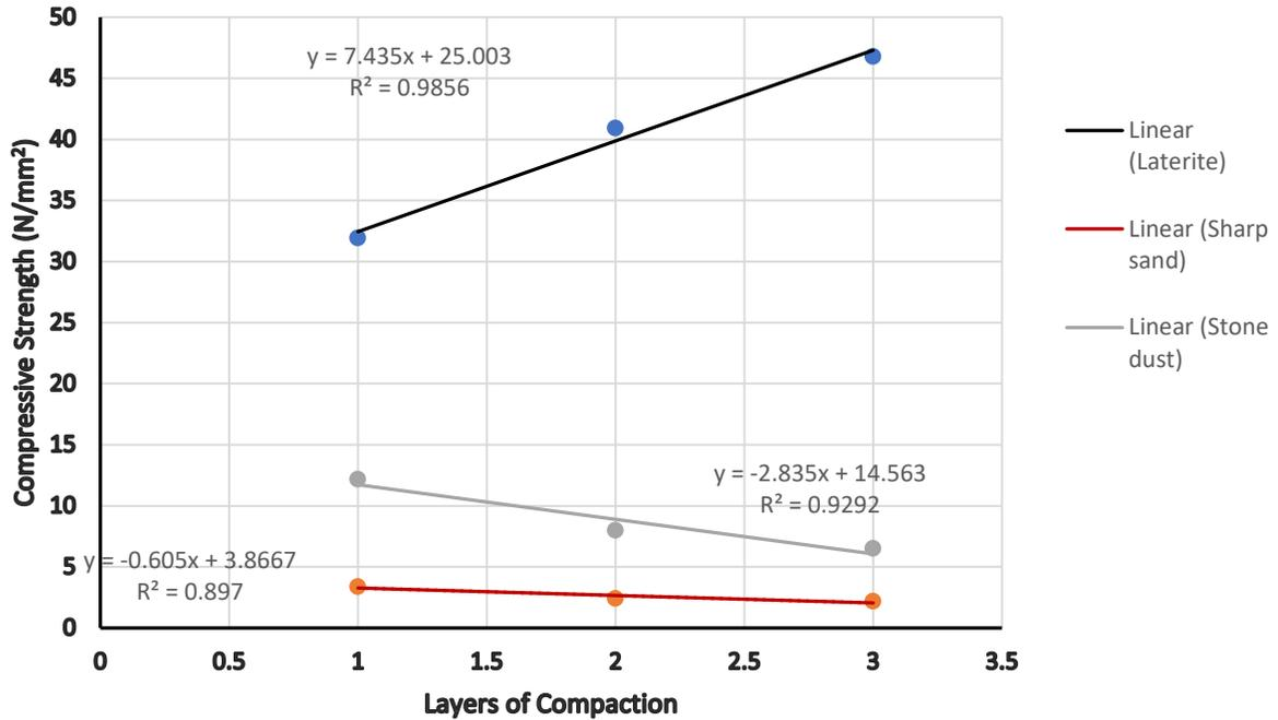
Figure 2: Variation of Compressive Strength with Compaction
