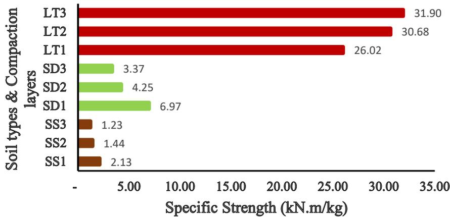
**Figure 3:** Effect of Soil Type and Compaction on Specific Strength of Eco-bricks
