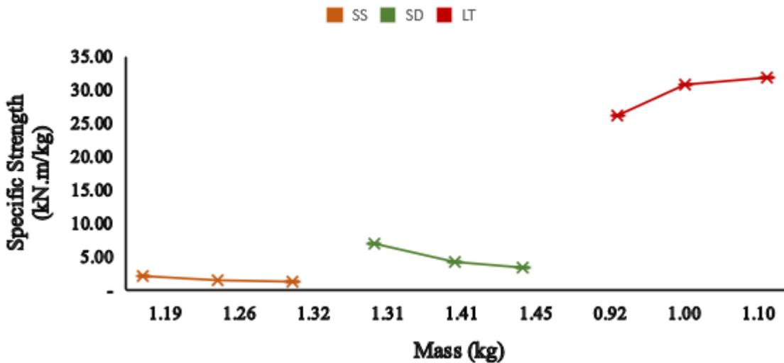
**Figure 4:** Specific Strength of Eco-bricks as a Function of Soil Material Mass
