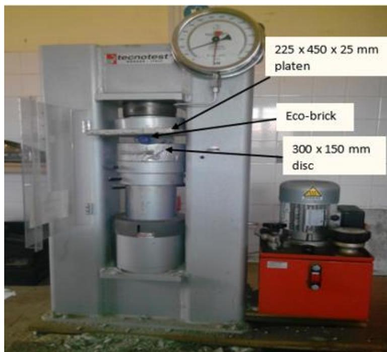
**Figure 1:** 750 ml Bottle Brick under Compression Load
