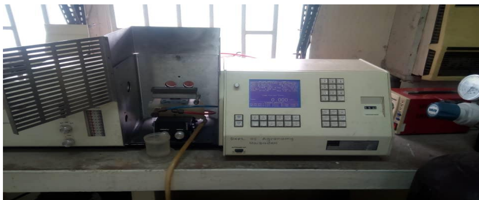
Figure 1: Atomic absorption spectrophotometer used for analysis
