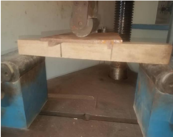
Figure 1: Four Point Bending Test Setup
