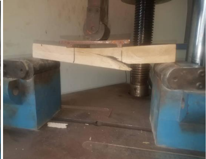
Figure 2: Failure Mode of Bending Specimens Test
