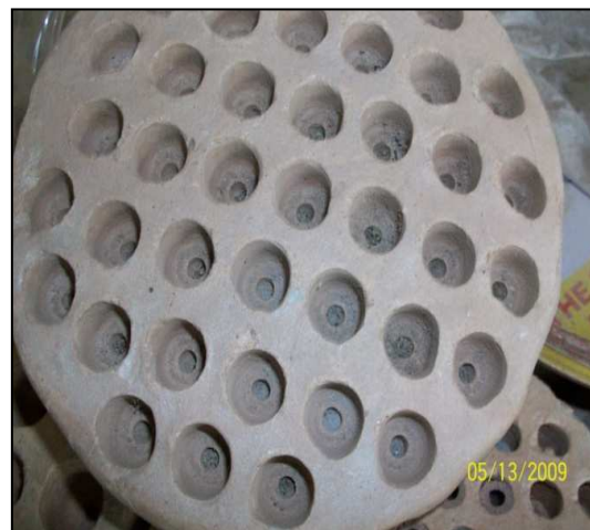
Fig. 5: Mould for bead casting
