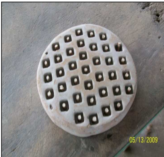
Fig. 9: Mould with cassava leaf stalks stuck into them
