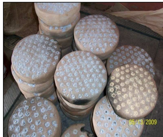
Fig. 11: Moulds filled ready for firing
