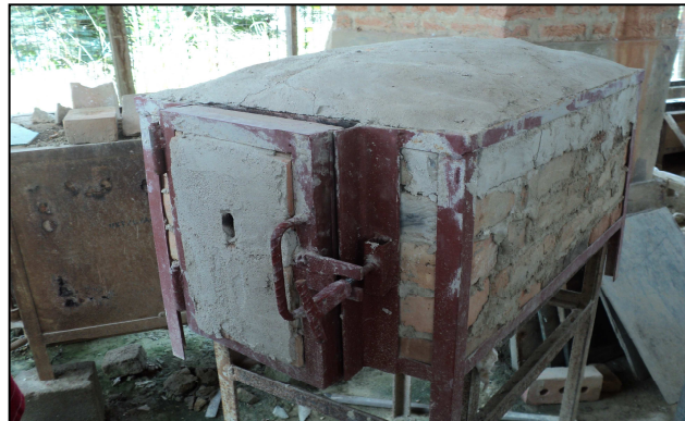
Fig. 2: Kiln for firing beads
