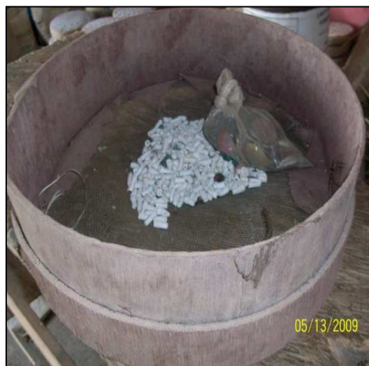
Fig. 8: Sieve for sieving the pounded glass
