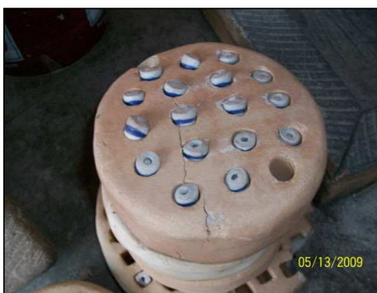
Fig.14: The newly cast beads in their moulds
