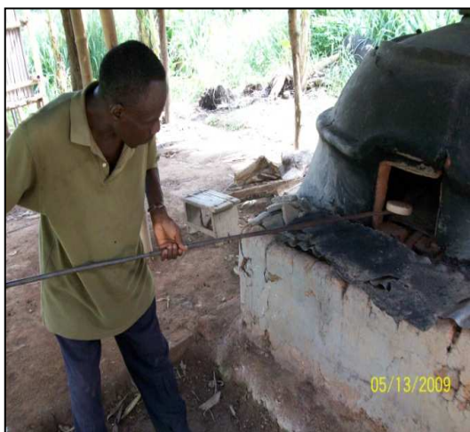
Fig. 13: Packaging mould into kiln Courtesy of Mr. Asumadu, beadmaker at Daabaa
