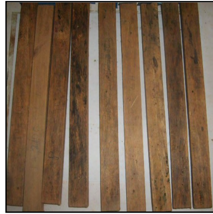
Plate 5b: Pyrinex 48EC-treated celtis stakes after 20-week field exposure
