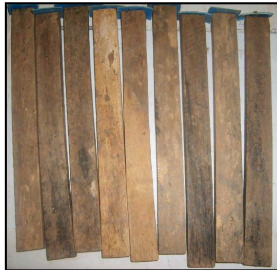
Plate 2b: Celtis control (untreated stakes) after 20-week field exposure showing some signs of damage including discolouration.
