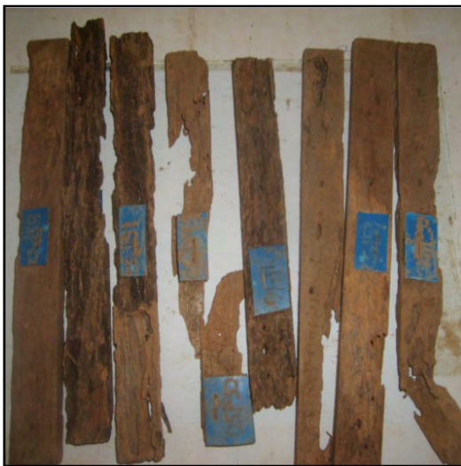
Plates 2a: Ceiba untreated (i.e. control) stakes after 20-week field exposure showing signs of damage
