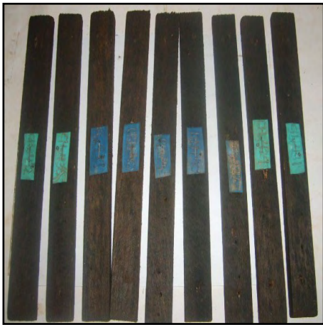
Plate 3a: CCA-treated ceiba stakes after 20-week field exposure
