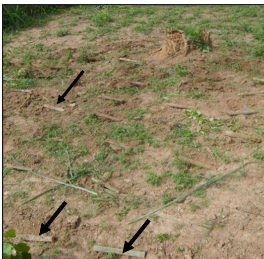
Plate 1: Test field showing stakes buried in the top soil for Accelerated Durability Test
