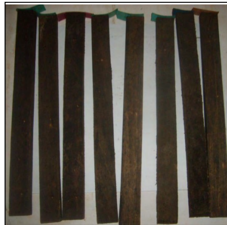
Plate 4b: Creosote-treated celtis stakes after 20-week field exposure
