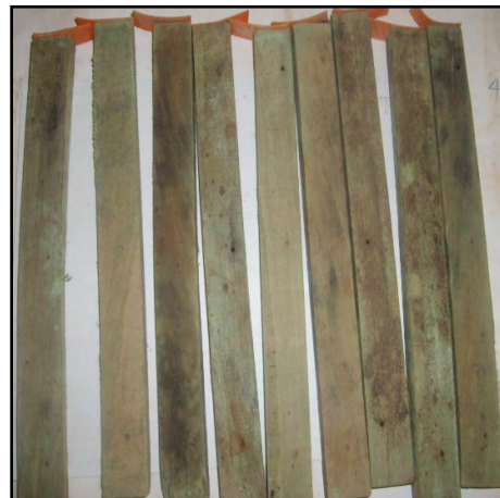
Plate 3b: CCA-treated celtis stakes after 20-week field exposure
