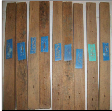
Plate 5a: Pyrinex 48EC-treated ceiba stakes after 20-week field exposure
