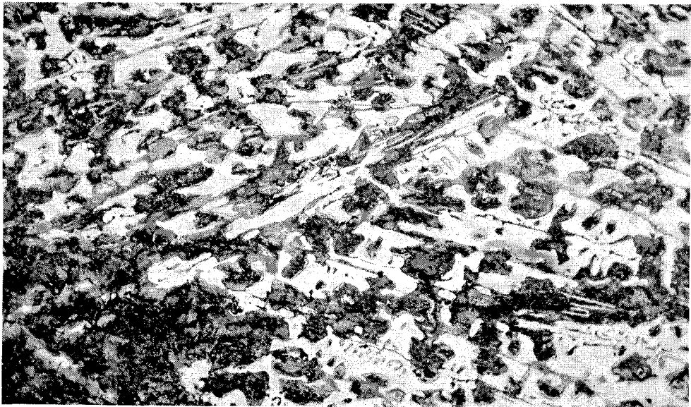
Plate 3. Microstructure of sample C consisting of fine lamellar pearlite and ferrite in a matrix of cementite ( Fe_3C ), with the latter phase accounting for about 60% of the total structure (200X)
