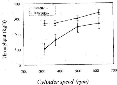
Fig. 1: Relationship between throughput and cylinder speed. Error bars represent the standard error of the mean.
