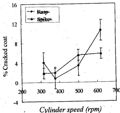
Fig. 3: Relationship between percentage of split bean and cylinder speed. Error bars represent the standard
