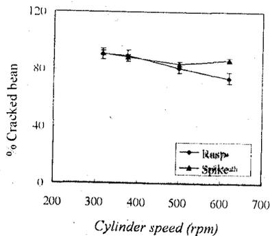
Fig. 4: Relationship between percentage of undamaged bean and cylinder speed. Error bars represent
