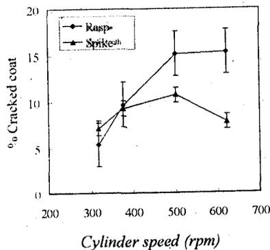
Fig. 2: Relationship between percentage of seed-coat crack and cylinder speed. Error bars represent
