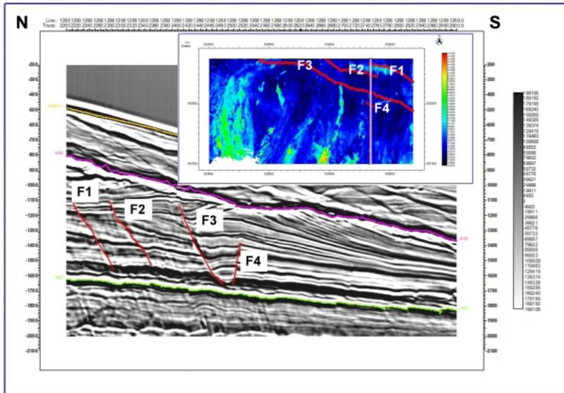
Figure 17: Seismic Inline showing major interpreted faults in section
