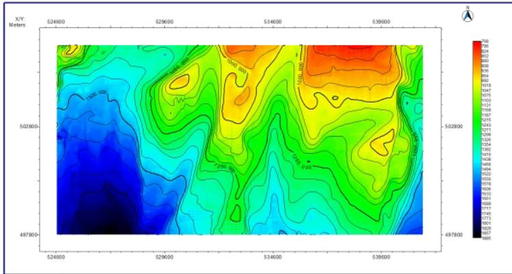
**Figure 11:** Depth/morphology map for horizon H1
