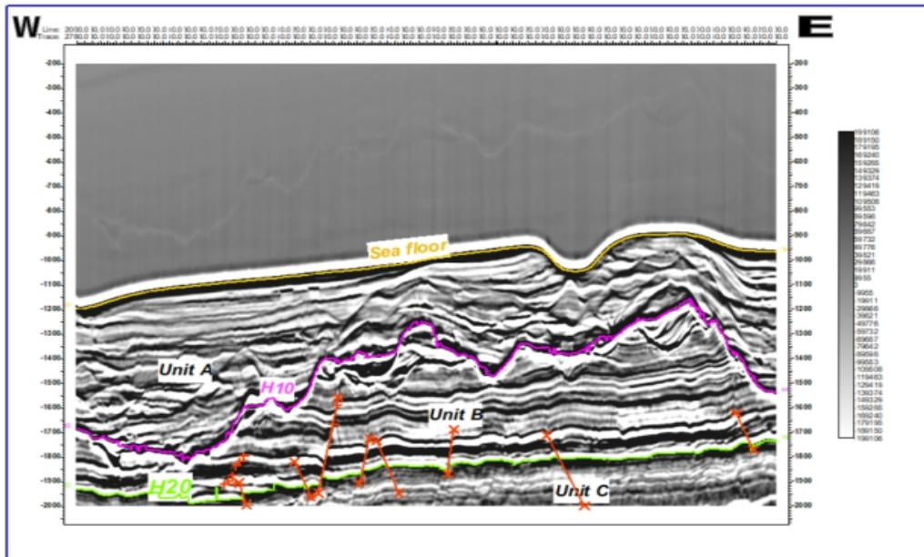
Figure 2: Crossline showing various units
