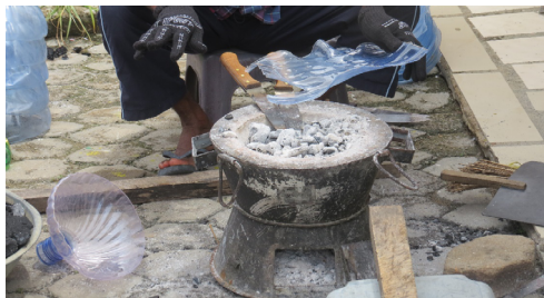
Figure 4: Post-consumer plastics being shaped.
