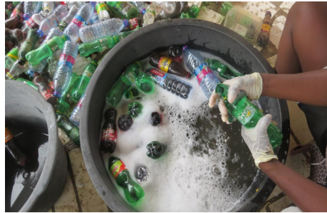
Figure 2: Washing of post-consumer plastic waste
