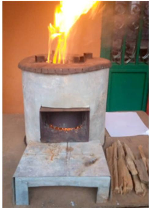
Figure 3.5: Combustion on TLUD Principle
