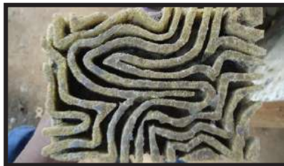
Fig. 10: Stamp E foam block for Fent E fabric
