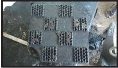
Fig. 6: Stamp a wooden block for Fent A fabric
