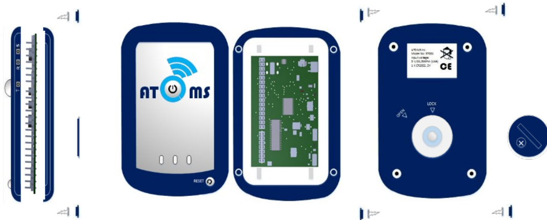
Fig.13: Exploded view of sensor-cluster microcontroller device
