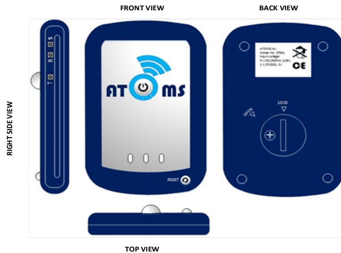
Fig. 12: Sensor-cluster microcontroller device packaging
