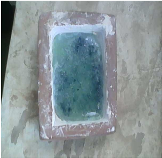
Fig. 11: Shrunken tile (120 Mesh fired at 1180°C)
