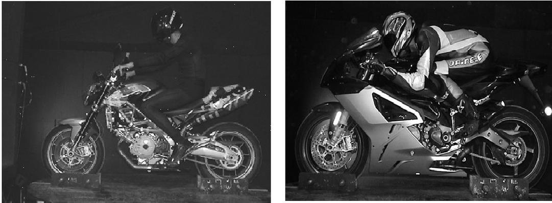
**Fig. 2 :** Motorcycles used in the tests: sport touring naked motorcycle (left); high performance sport bike (right); note the differences between driver postures (photos published courtesy of the Piaggio group)
