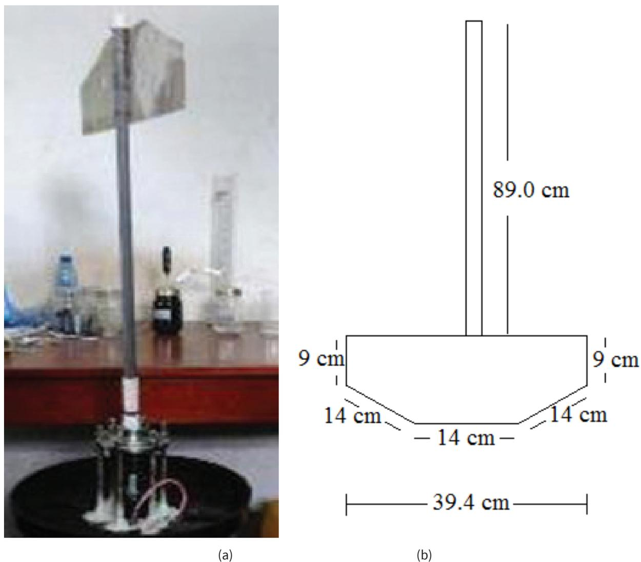
Fig. 3: Motorized stirrer with schematic diagram
