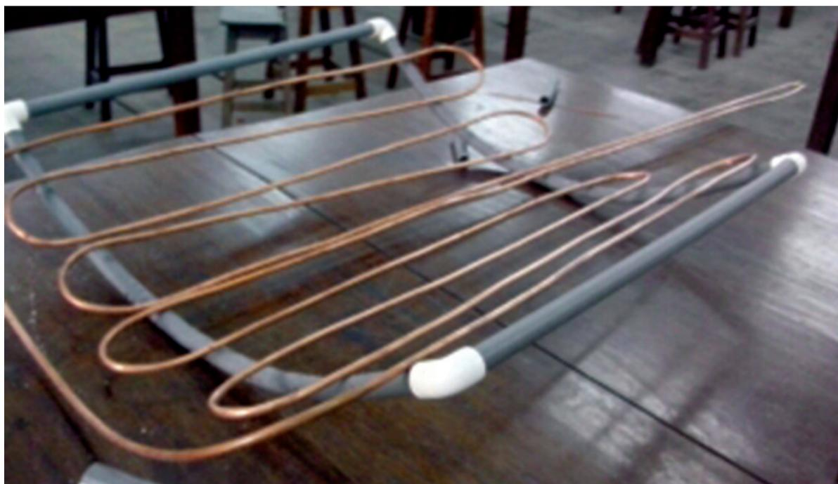
Fig. 2: Copper tubing heat exchanger
