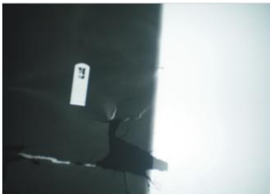
Figure 1: An image of a section of a lead apron with Tear and crack defects
