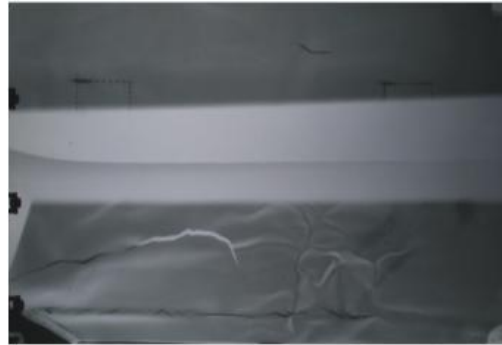
Figure 3: An apron with crack and tear defects
