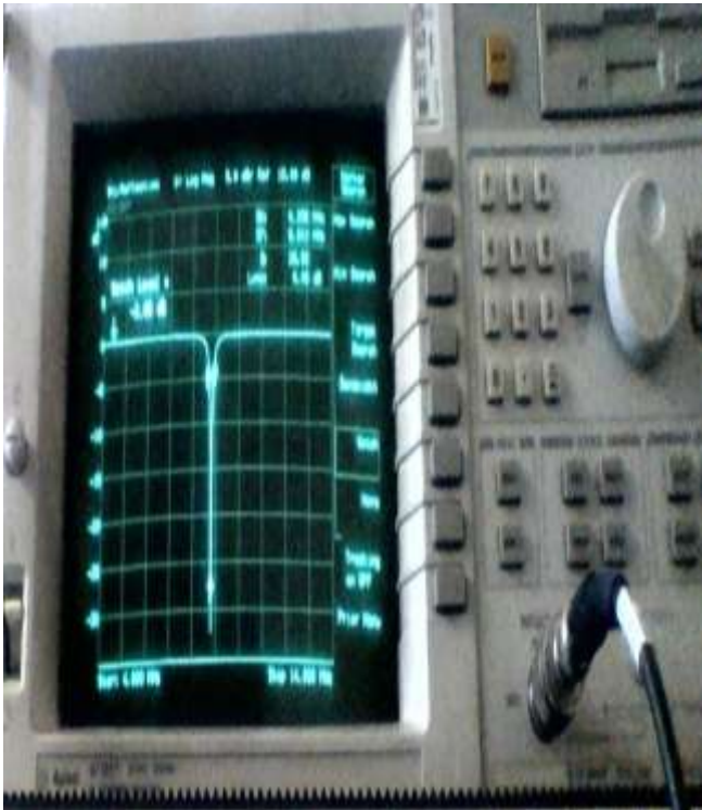
Figure 7: Image display of an RF network analyser used for this experiment. A coaxial cable connecting the RF probe to the reflection mode of the network analyser is also displayed. On the upper left edge is a display of the resonant frequency and the corresponding attenuation. The lower marker represents the maximum attenuation.
