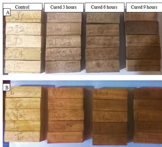
Fig. 6: A: 10 years and B: 15 years Gmelina arborea wood impregnated with lactic acid and cured at different time
