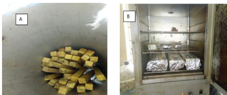
Fig. 1: (A) Wood loaded in the Impregnation Chamber (B) Curing Processing in Oven
