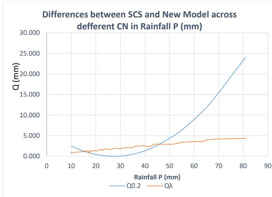
**Figure 1: Runoff difference curve graph of Kainji dam.**
