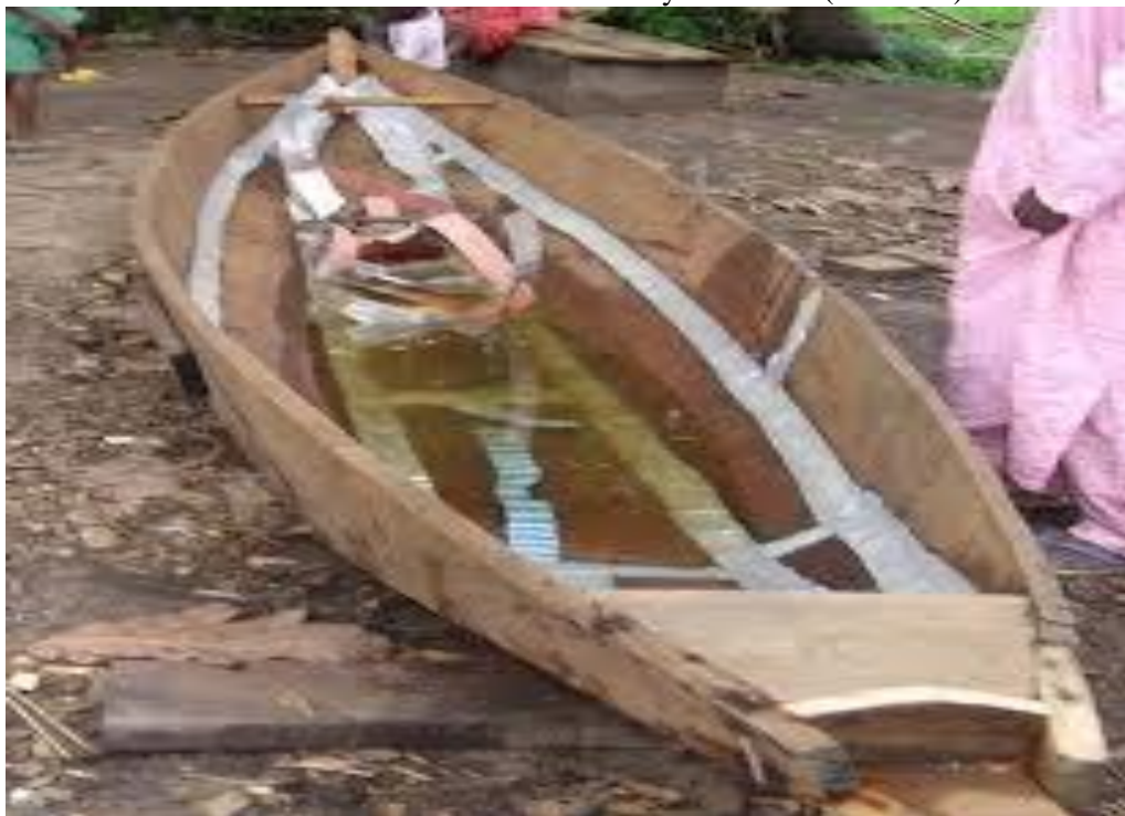
Plate 6: A newly constructed planked Canoe with strips of galvanized iron aluminum
