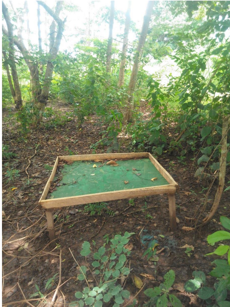
Figure 1. Littertrap erected at the centre of a sample plot in the Terminalia superba plantation
