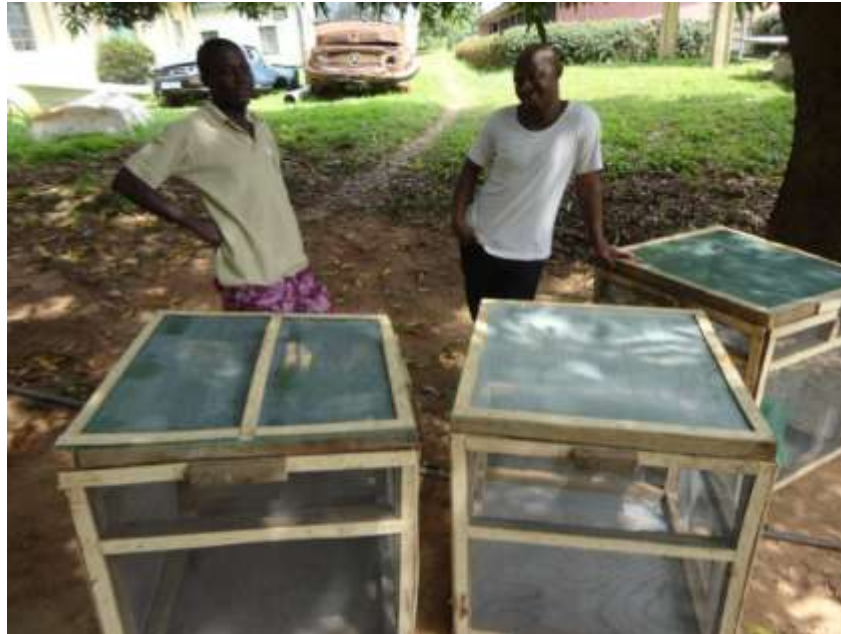
Plate 1: Cages constructed in this experiment for the culture of the mudfish Clarias gariepinus in River Benue
