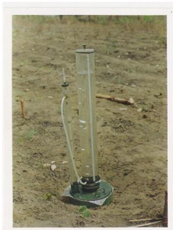
**Figure 2** Tension infiltrometer in operation
