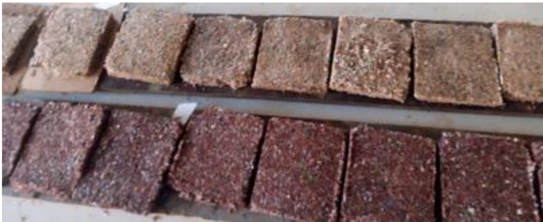
Plate 14: Wood plastic boards produced K. senegalensis and G. arborea spread to dry
