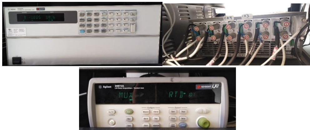
Fig 2. Machines analysis of I-V curve (a)Data logger N3300A, front face and (b) bike side, Data acquisition , Keysight 34972A.
