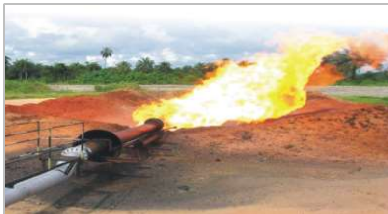
Plate 1: A typical horizontal/ground gas flaring jet [22]
