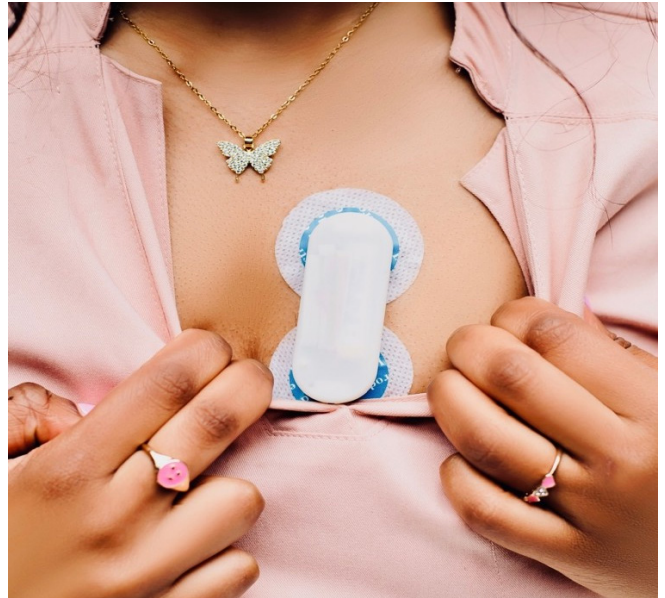
Figure 2: Image demonstrating the wearable ECG device with electrode adhesives
