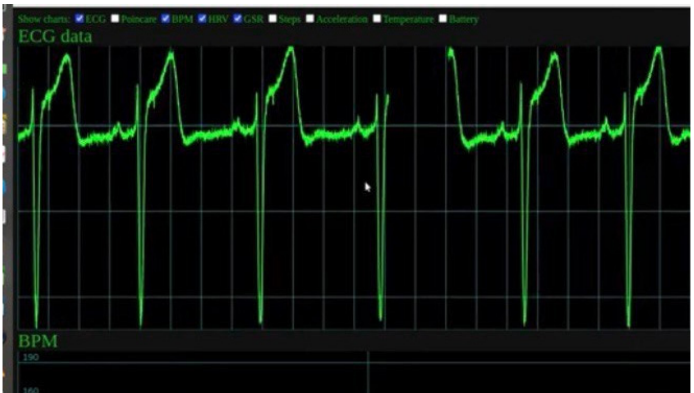
Figure 3: Dashboard showing real time ECG data, BPM, HRV, GSR, Steps, Acceleration and Temperature (BLE data transmission from hardware to software interface)
