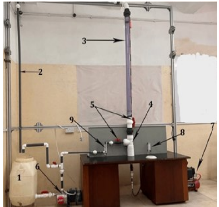
Figure 4 Two-phase flow experimental setup with 3mm test section with key components labelled 1–9; Note: 1=water reservoir, 2=0.5 in pipe, 3=bubble column, 4=air-water mixer, 5=valves, 6=water pump, 7=air compressor, 8=air flow meter, and 9=water flow meter
