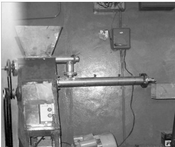
Figure 10 Food extruder 1. (LEGEND: A- Hopper, B- Feeding Conveyor, C- Extruder worm, D- Die Unit, E- Power train, F- Conveyor pulley, G- Extruder pulley, H- Extruder Housing, I- Control switch) (Fayose et al. , 2017)
