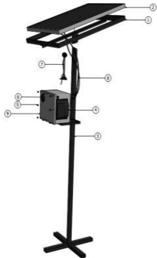
Figure 8 Solar powered audio based bird repellent system for rice fields (LEGEND: 1- Frame, 2- Solar panel, 3- Stand, 4- Charge controller, 5- Nut, 6- Speaker, 7- Camera, 8- Cable, 9- Adaptable box) (Arowolo et al. , 2022)
