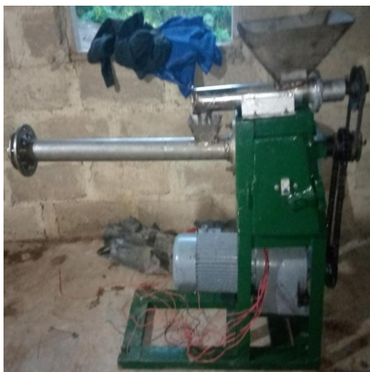
Figure 11 Fish feed extruder with extruded fish feed
