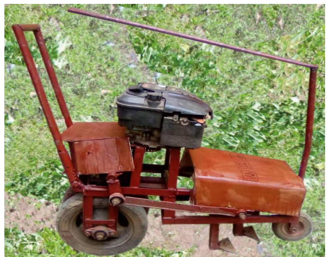
Figure 1 The (a) jab planter, (b) 3D view of rotary jab planter, and (c) rotary jab planter (Source: Fayose et al. , 2021)
