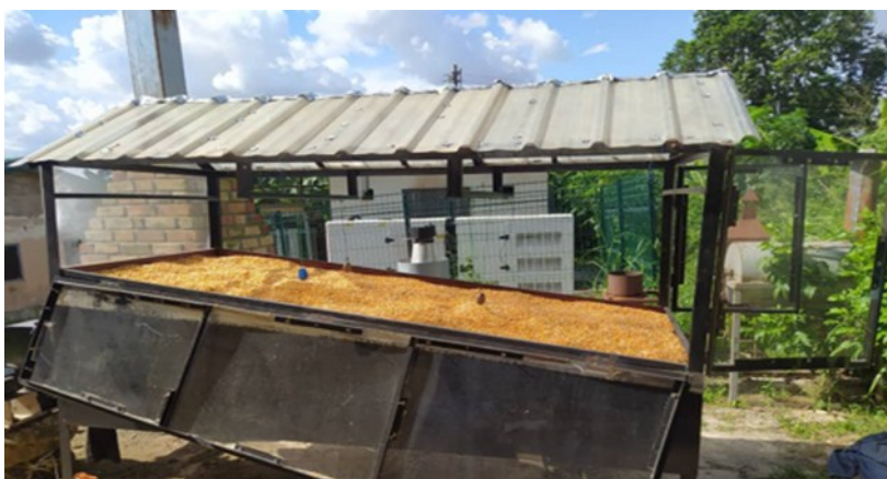
Figure 2 Experimental set-up of drying maize in the biomass-powered inclined bed dryer
