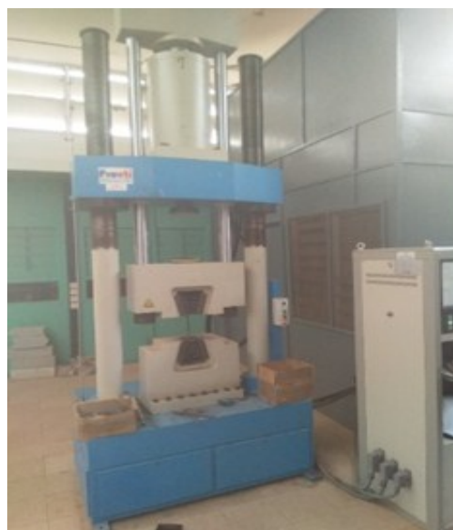
Figure 1 Setup for tensile strength analysis using PROETI: DI-CP/V2 tensile test machine
