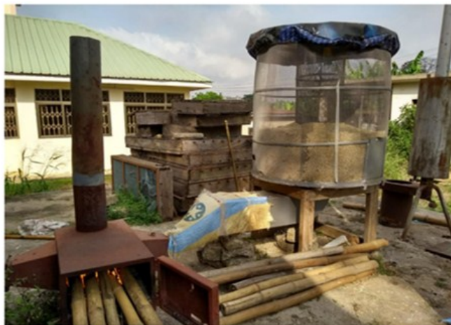
Figure 2 KNUST STR column dryer with the CAD model
