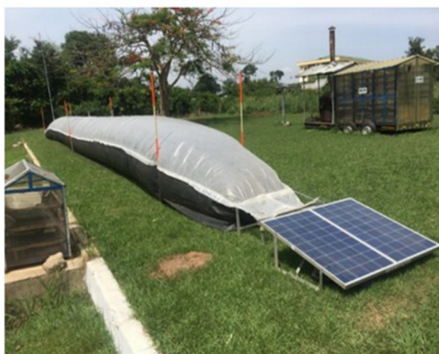
Figure 3 Solar bubble dryer setup at KNUST with an insert of its labelled components
