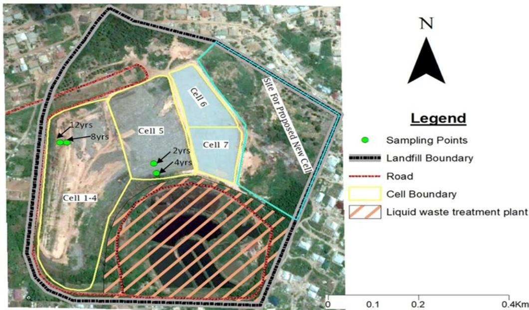
**Figure 1** Layout of Kumasi landfill and location of sampling points
