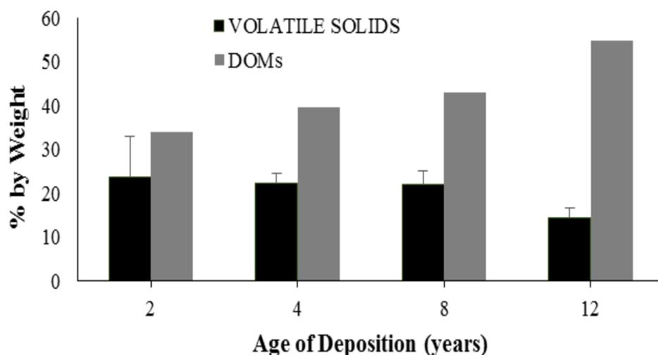
**Figure 4** Variation of volatile solids content and proportion of DOMs with the age of deposition of waste
