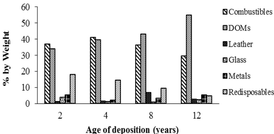
**Figure 3** Composition of landfill waste for different ages of deposition of waste
