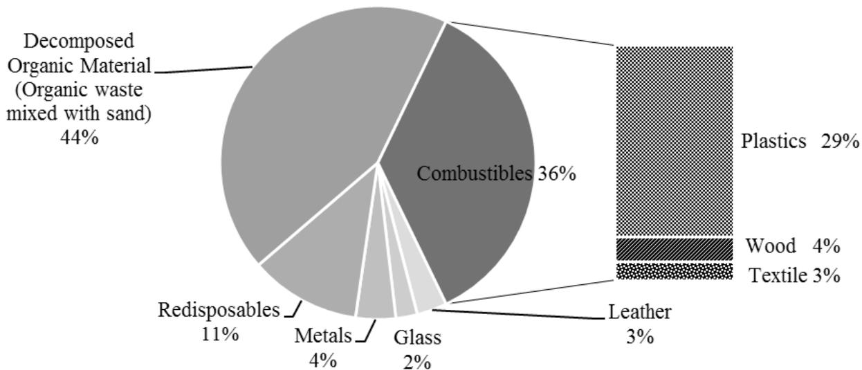
**Figure 2** Composition of excavated landfilled waste at the Kumasi landfill site
