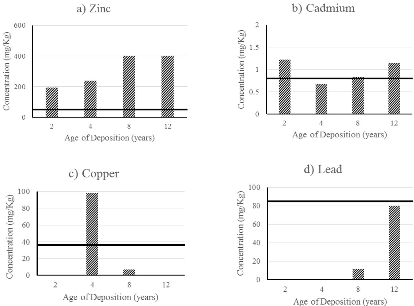
**Figure 5** Heavy metal concentrations in DOMs with the age of deposition of waste
