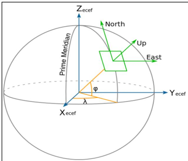
**Figure 1** Geodetic coordinate systems
