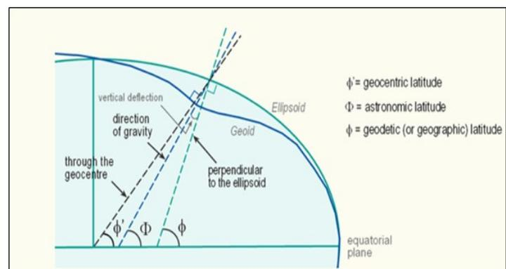
**Figure 2** Three different latitudes: the geodetic, the astronomic and the geocentric latitudes (Soler *et al.*, 2014)
