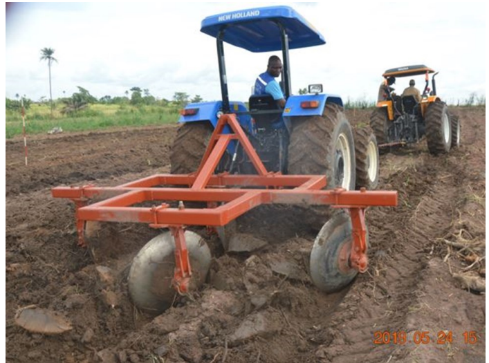
Plate 3 Tractors–dynamometer, implement mounted in tillage operation
