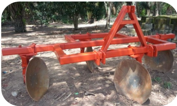
Plate 4 The fabricated fully mounted double row disc ridger ready for testing
