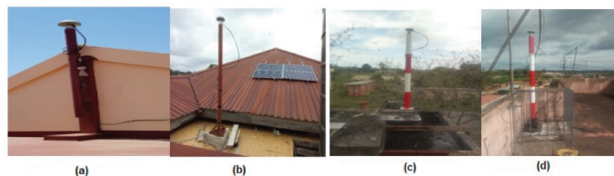
Figure 1 (a) Antenna mount of Spintex CORS, (b) Antenna mount of Adum CORS, (c) Antenna mount of Tarkwa CORS and (d) Antenna mount of Oda CORS.
