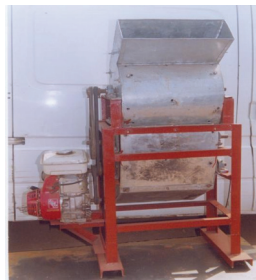
Figure 4 Automated cassava peeling system (Olukunle and Akinnuli, 2013)
