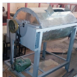
Figure 12 Peeler using sun and planetary mechanism (Adekunle et al. , 2018)
