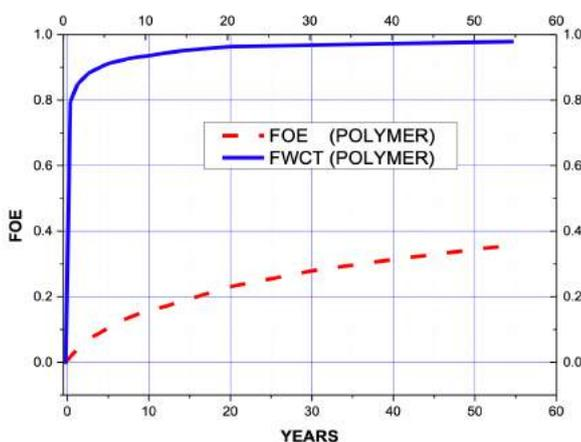
**Figure 5** Oil field recovery and field water cut over time using
