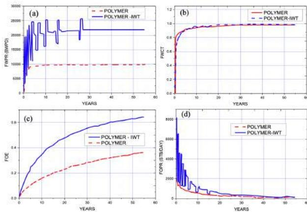
**Figure 14:** Comparison between the performances of the base case and production control case of the (a) water production rates FWPR, (b) water cuts FWCT, (c) oil recovery FOE, and (d) oil production rates FOPR
