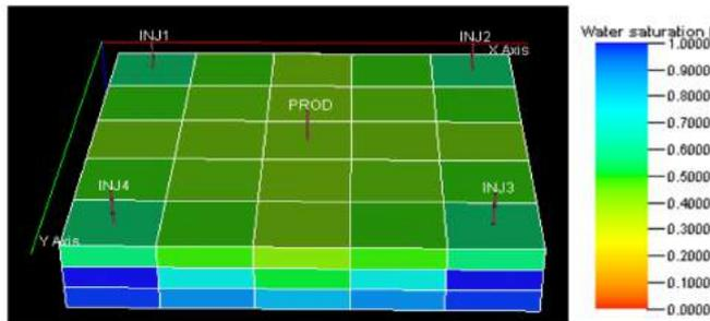
**Figure 4** Base case - polymer injection 3D model of remaining saturation of oil after a 55-year run
