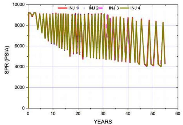
**Figure 16** Injection pressures of injector wells 1, 2, 3 and 4
