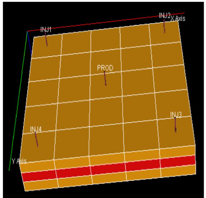
**Figure 1** The reservoir model of the 4 injection wells and 1 producer well for a 5-spot pattern
