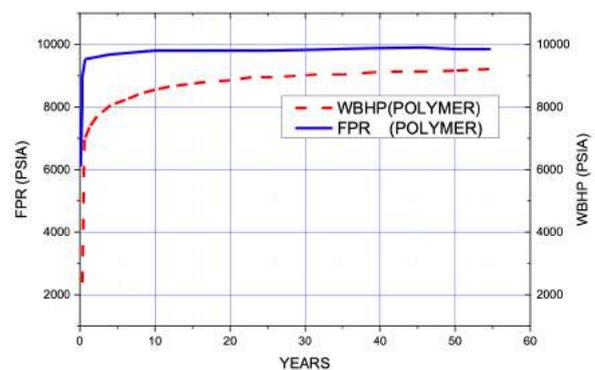
**Figure 7** Average pressure and well bottomhole flowing pressure at the production well (PROD)
