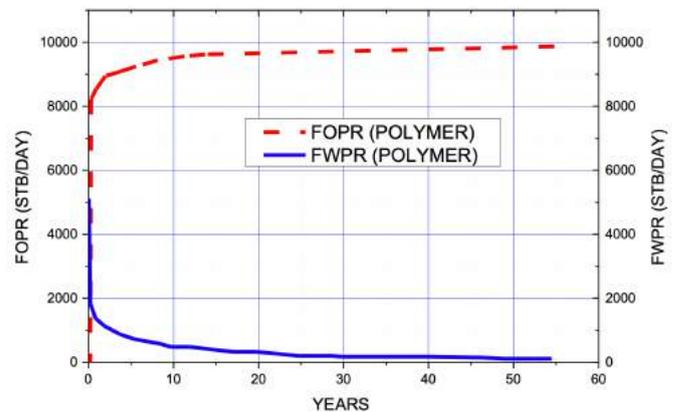
**Figure 6** Oil production rate and field water cut over time using polymer injection
