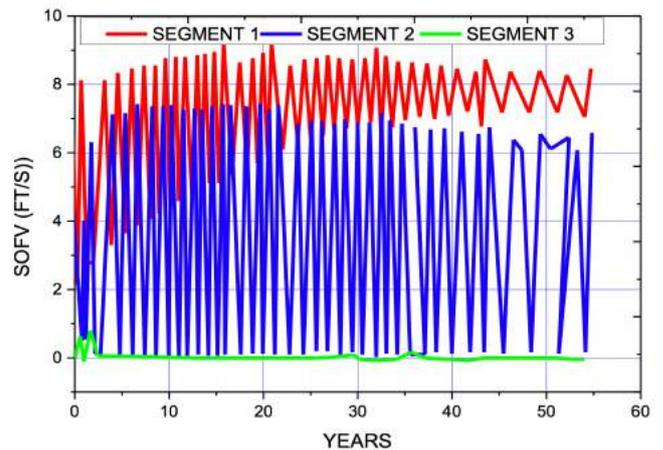
**Figure 17** Segment oil flow velocities for the production well
