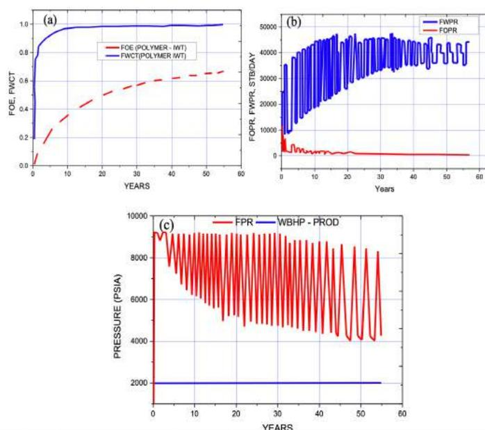
**Figure 19** (a) Oil recovery and field water cut versus time, (b) the oil and water production rates over time, and (c) reservoir pressure and production well bottom hole pressure
