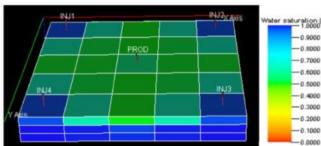
**Figure 8** The production control case 3D model of the remaining saturation of oil after a 55-year run
