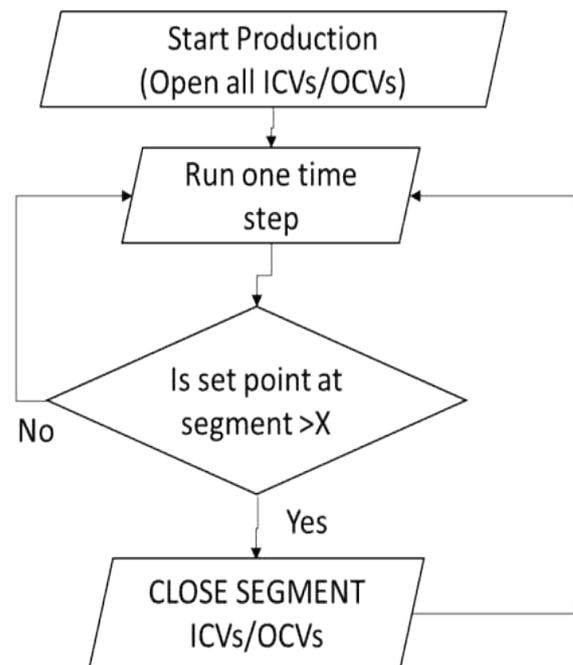
**Figure 3** The reactive control strategy for either injection and production control or the injection of polymer using IWT
