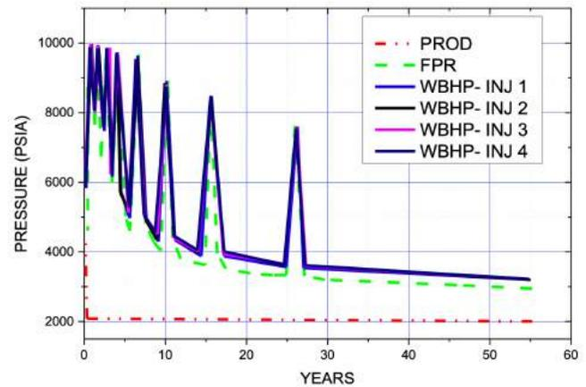
Figure 13 Pressures at the well injectors and producer
