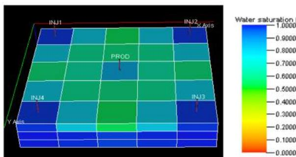
**Figure 15** The injection control case 3D model of the remaining saturation of oil after a 55-year run
