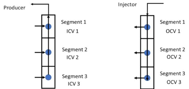
**Figure 2** Implementation of the IWT in the simulator
