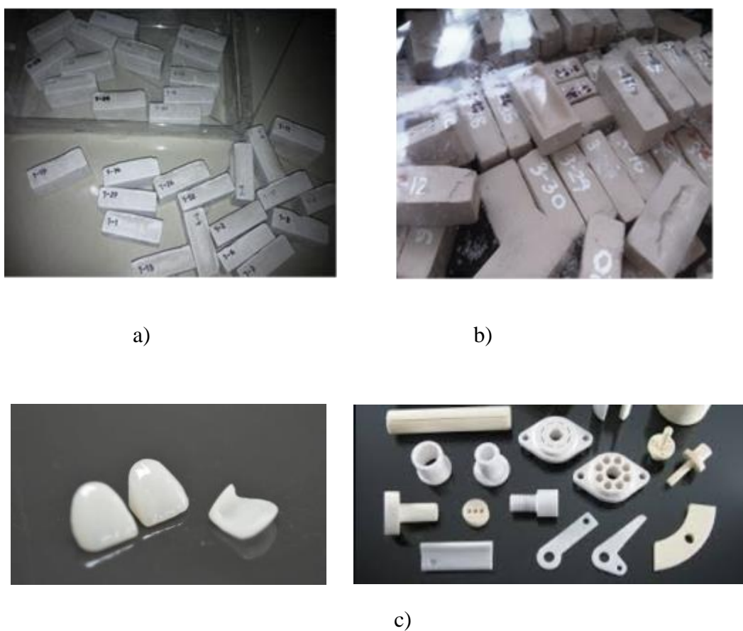
Scheme 3. Porcelain samples a) before firing, b) after firing, and c) porcelain applications
