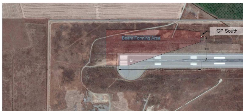
Fig.7. Proposed position of glide path and beam-forming zone
