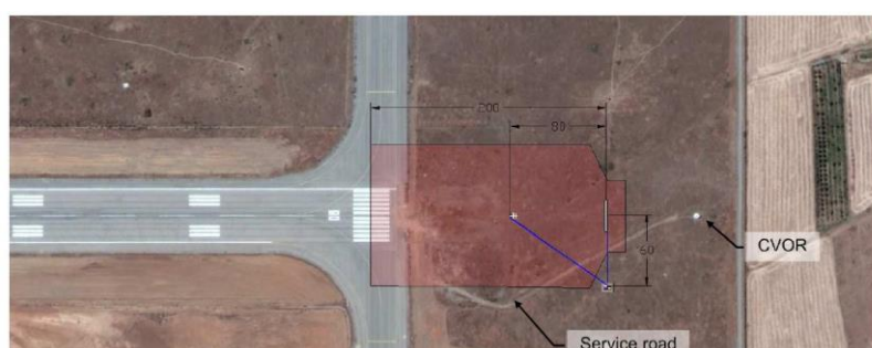
Fig.6. Lay-out of the localizer
