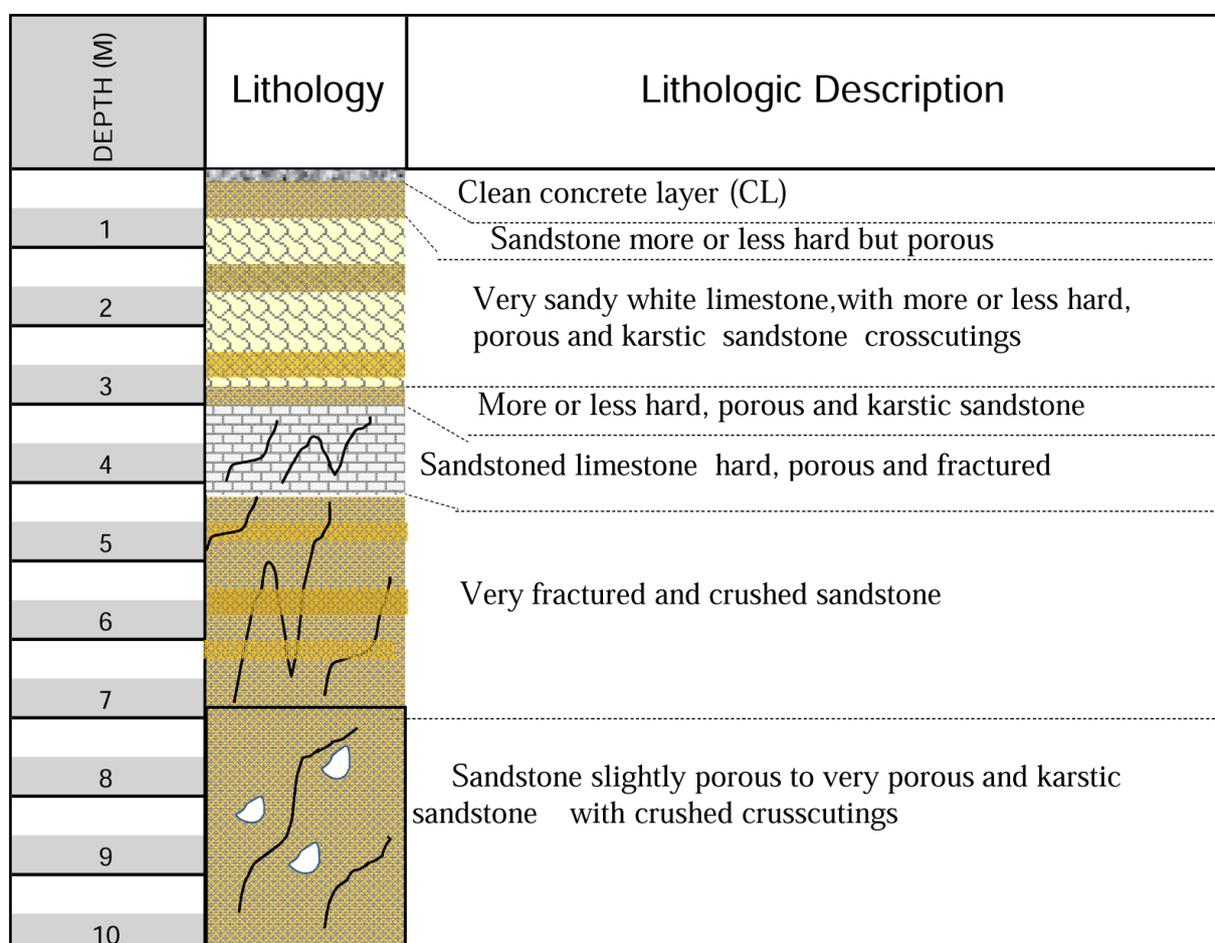
**Fig.2.** Lithological section of the study area (realized on the pile N° 3)
