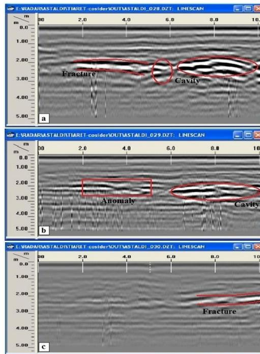
**Fig.8. a, b and c** Transverse radargrams with 45 cm, 2 m, and 4 m, respectively of the edge for excavation of foundation P3
