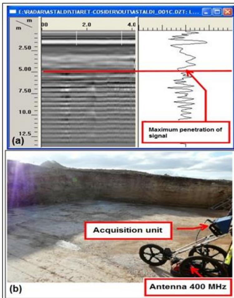
**Fig.5.** (a) Limit penetration of the signal for GPR. (b) Methodology of GPR
