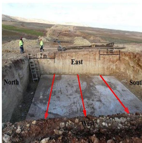
**Fig.6** Photograph showing the orientation of GPR profiles
