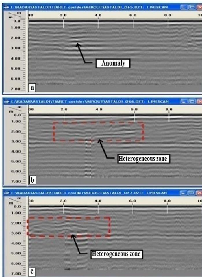
Fig. 11. a, b and c Profile radargrams for excavation of foundation P10, for the profiles N°1, N° 2, and N°3 respectively
