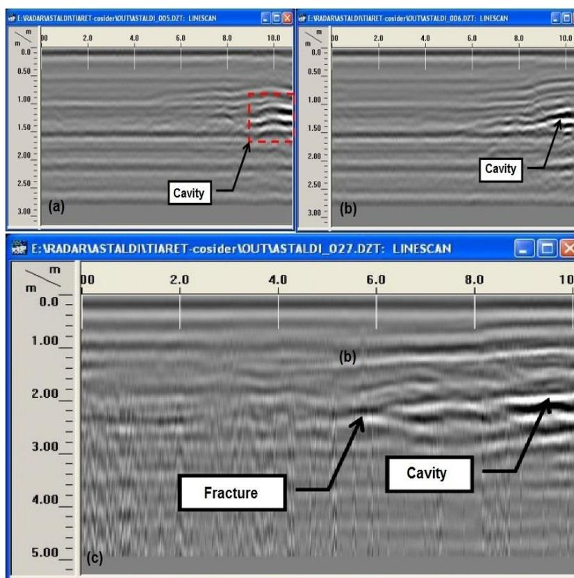
**Fig.7. a and b** Longitudinal axis profile radargrams with antennas 400 and 200 MHz. **c** Longitudinal radargram N°3 for excavation of foundation P3
