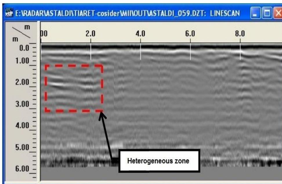
**Fig. 10. a** Profile radargram N° 3 for excavation of foundation P6
