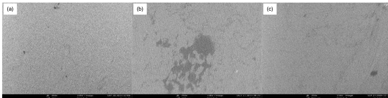
Fig.4. Scanning Electron Microscope (SEM) Images for a) fresh b) uninhibited and c) inhibited Aluminium samples
