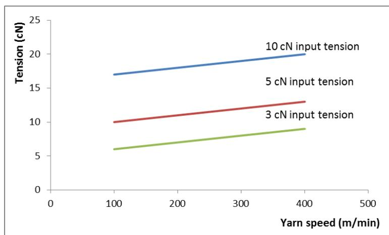
**Fig.4.** Variation of output tension with different input tension and speed
