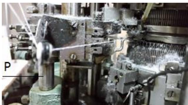
**Fig.2.** Short fibers in cotton deposited on circular knitting machine devices.
