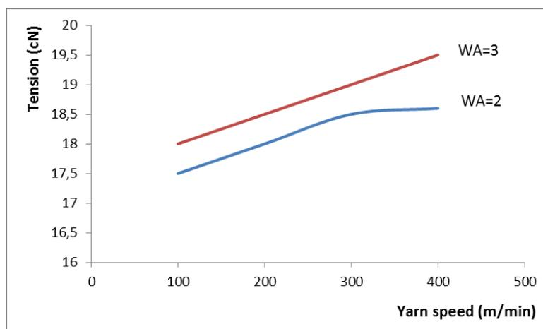
**Fig.5.** Variation of output tension at different yarn wrap angle
