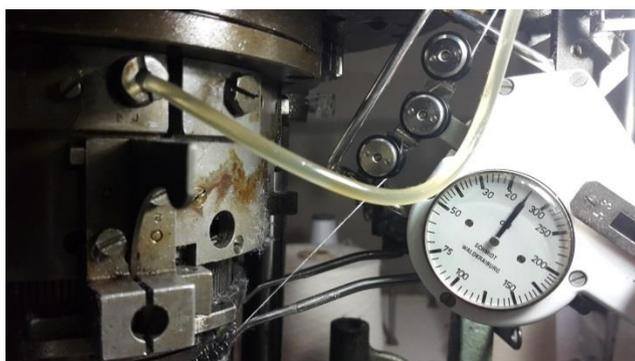
**Fig.3.** Input and output tension of yarn during production.
