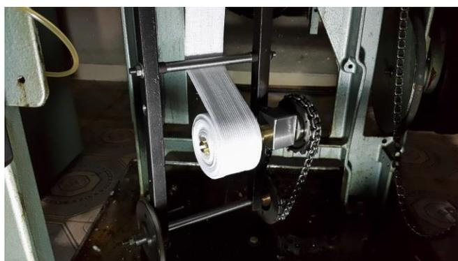
**Fig.1.** Circular knitting machine Bentley komet transformed to produce continues simple jersey fabric. Photo, Ali Bey H, Algiers
