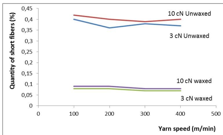
**Fig.7.** Amount of short fibers generated with different tensions, waxed and unwaxed yarns, (needle gauge 14, A 3 radian)
