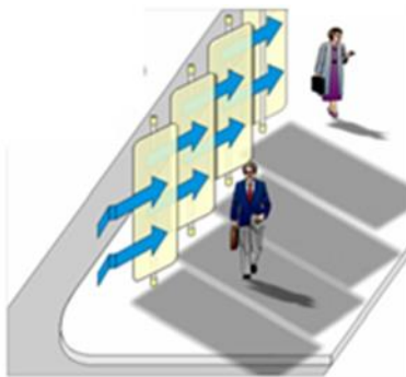
Fig.1. Panels used to create shade and channel the flow of air [5]
